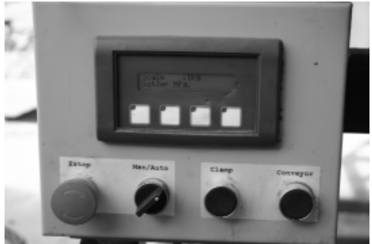
Adjust the levels for the appropriate bag weight. The red emergency stop is the first button on the left of the control panel.
