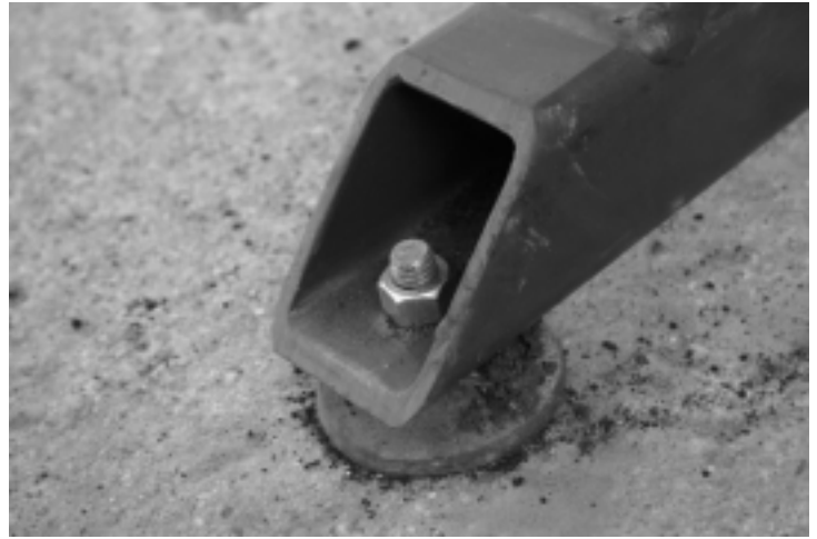
To level the machine adjust the nut on the foot of each support appropriately.
