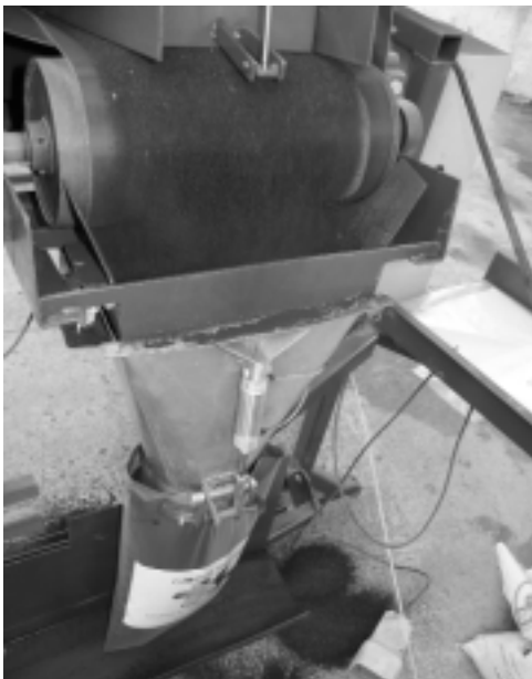
Check air operated drop gate for free movement.
