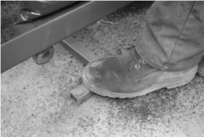
The height of the pan that holds the full bags can be conveniently adjusted with a foot pedal.
