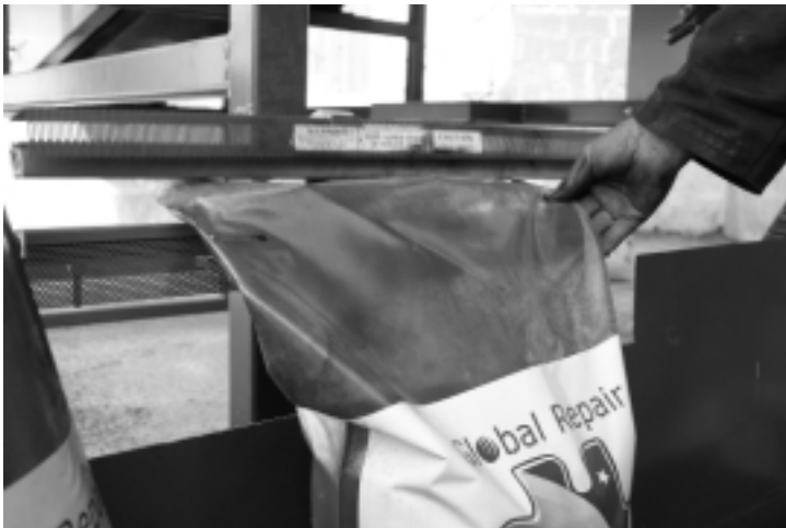
Do not place fingers in between heat clamps. Heat resistant gloves may be required for additional safety.
