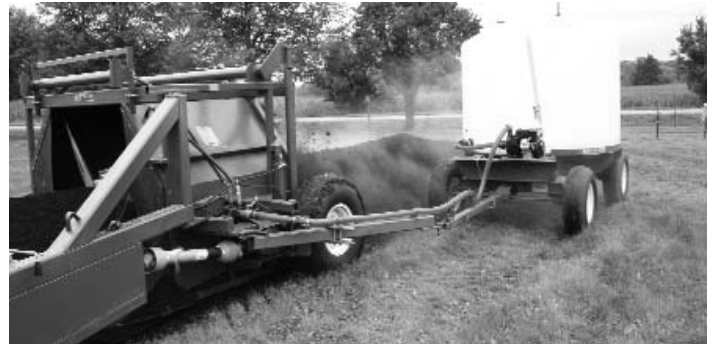
See Water Wagon and Windrow Turner applying water.
